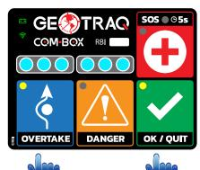
Vehicle B is being overtaken: Lights BLINK BLUE CONFIRM OVERTAKING WITH BLUE BUTTON ! (will allow overtaking at the first safe place)
